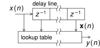
**Figure 3: A generalization of Fig. 2 to a continuous-time output. Here the nonlinearity  $\mathbf{N}(\cdot)$  maps the  $2^N$  distinct  $N$ -vector address inputs  $\mathbf{x}(n)$  onto the  $2^N$  distinct standard unit vectors  $(0 \dots 010 \dots 0)^T$  of length  $2^N$ . This unit vector selects a waveform segment from vector  $\mathbf{w}(t)$  to be the output  $y(t)$  in clock interval  $n$ .**
