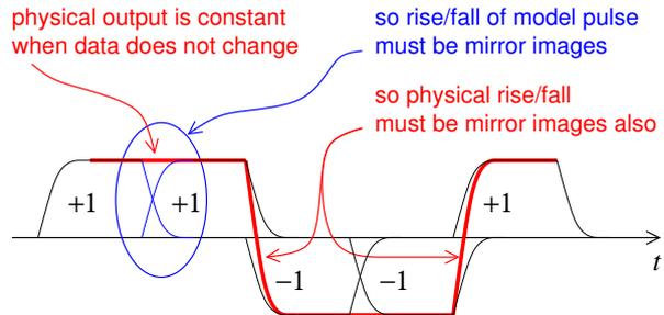
Figure 1: NRZ data with asymmetric transitions can never be expressed as  $\sum_n x(n) h(t - nT)$ , as  $\pm 1$  binary data  $x(n)$  LTI modulating a model pulse  $h(t)$ . Asymmetry implies nonlinearity.
